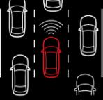
CTS assists to maintain a constant distance between your vehicle and a vehicle ahead at a preset vehicle speed without you having to use the accelerator or brake pedal. It also assists the driver to keep steer the vehicle within the lane lines.
